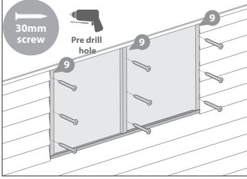
Fix the window strips to the two pieces of framing that sit alongside the outside edges of the window with 3x30mm screws for each strip.
