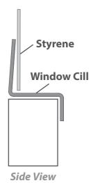
Place the plastic window cill onto the Window Panel and silicone in place as shown on both diagrams to the left.
