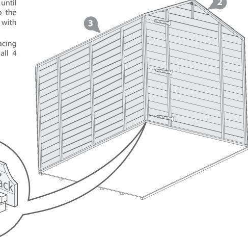
Fix the corners with 50mm screws as shown in diagram.
