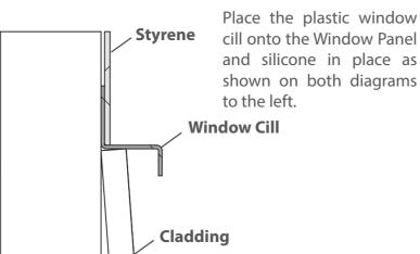
Fit the styrene sheets on top of the window cill.
