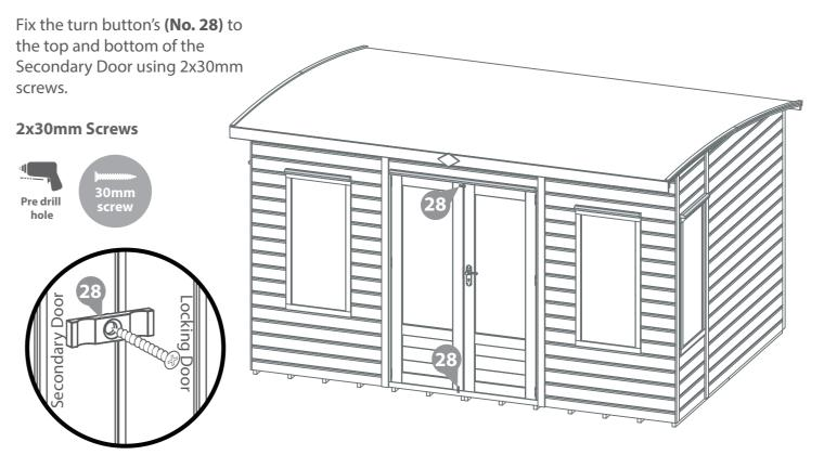
\*These turn buttons help keep your doors straight during high and low levels of moisture content in the air.
