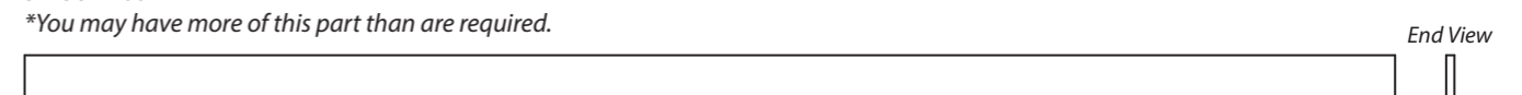
20 Fascia - 12x60x2000mm QTY 6** S1260-2000mm *You may have more of this part than required.
