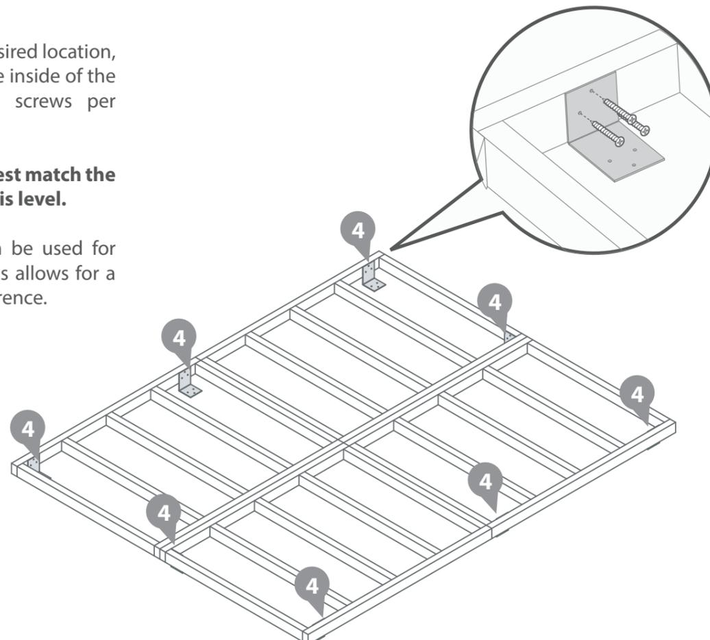
**IMPORTANT: Pre-drill before fixing screws.**
