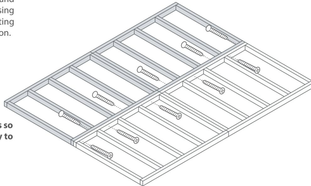
**IMPORTANT: Pre-drill before fixing screws.**
