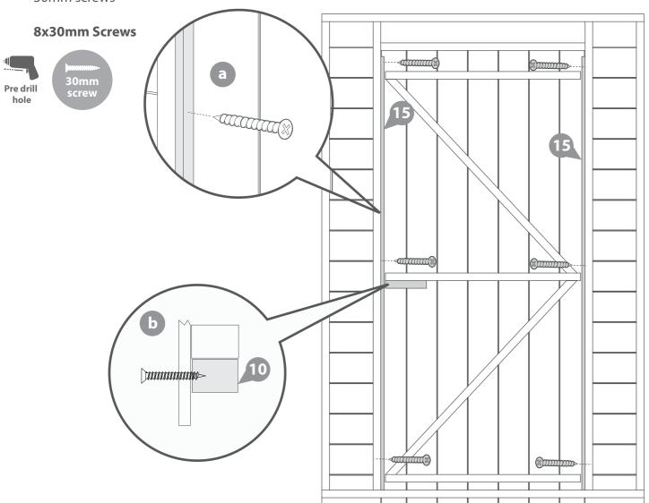
IMPORTANT: Pre-drill before fixing screws.
