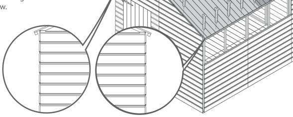
IMPORTANT: Pre-drill before fixing screws.
