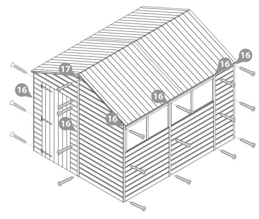
IMPORTANT: Pre-drill before fixing screws.
