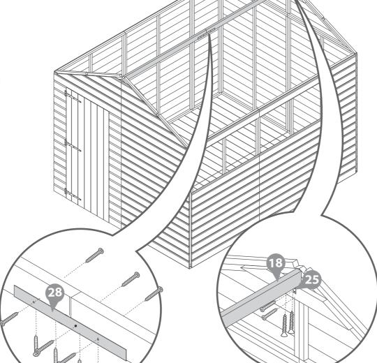
IMPORTANT: Pre-drill before fixing screws.
