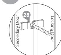
**IMPORTANT:** *Pre-drill before fixing screws.*
