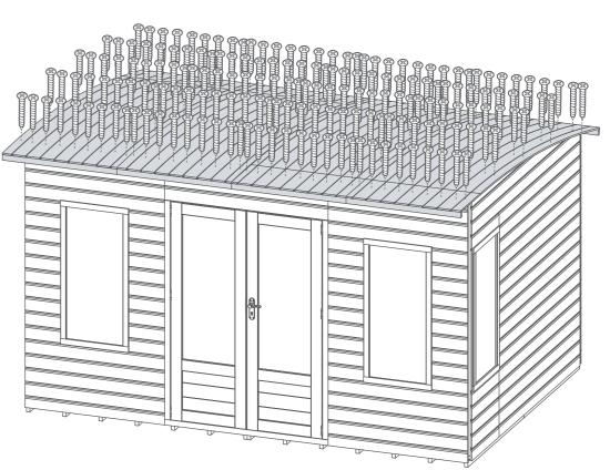
**IMPORTANT:** Pre-drill before fixing screws.
