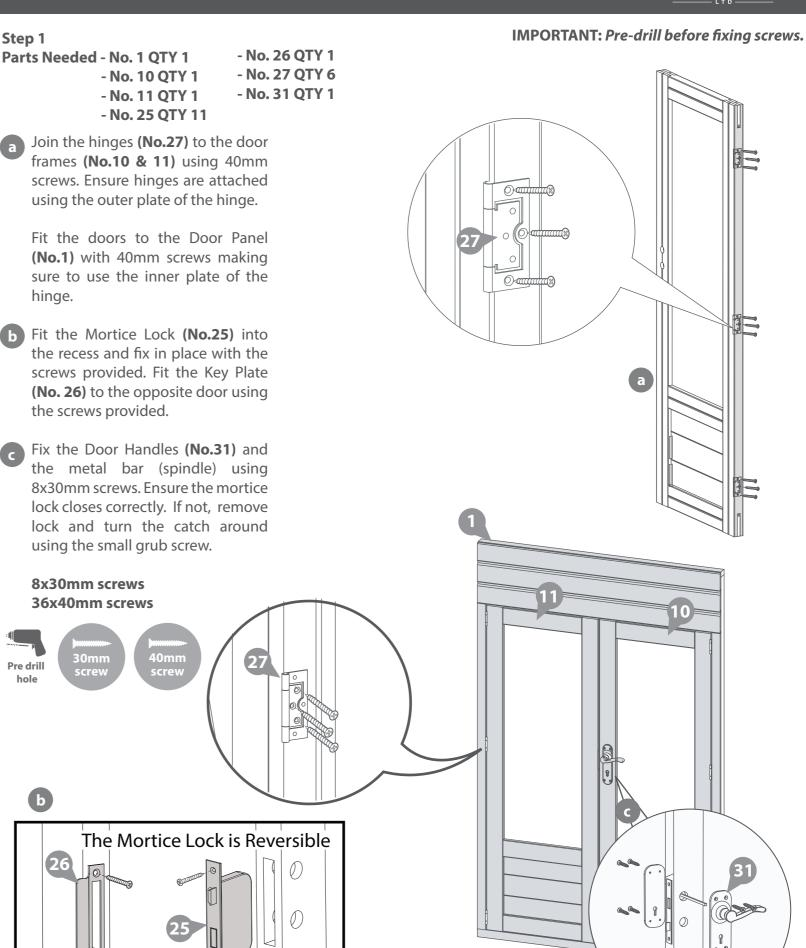
IMPORTANT: Pre-drill before fixing screws.
