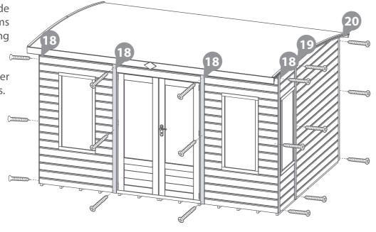
IMPORTANT: Pre-drill before fixing screws.
