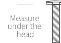
To identify the fixings required for each step use a measuring tape.
