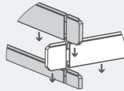
Following the method shown in the illustration, lay the next layer of boards (**No. 2, 7 & 8**) onto the log cabin
