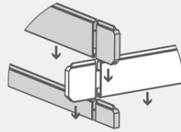
**\*Ensure that the boards are level and flush with each other as you lay each one.**
