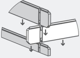
Following the method shown in the illustration, lay the next 6 boards (**No. 2, 3 & 5**) onto the log cabin to create your third level.
