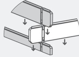
Following the method shown in the illustration, lay the next 6 boards (**No. 2, 3 & 5**) onto the log cabin to create your second level.
