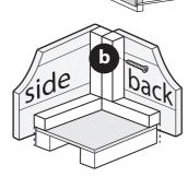
IMPORTANT: Pre-drill before fixing screws.
