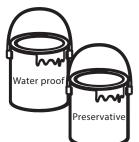
Once your garden building has been installed it will need to be treated within 14 days (weather permitting) and annually to prevent the timber from deteriorating and to waterproof it. This is required to maintain the anti-rot guarantee.
