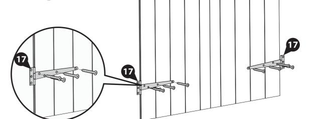
Align each door (No. 6) into the door gap and secure at either side using 3x30mm screws per t-hinge (No. 17).
