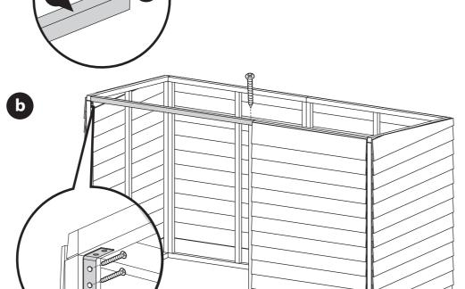
IMPORTANT: Pre-drill before fixing screws.
