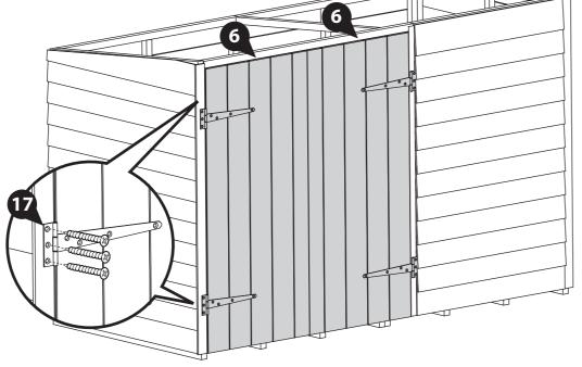
IMPORTANT: Pre-drill before fixing screws.
