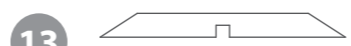
13 Underside Support B - 40x40x800mm QTY 1 F4040-G-800mm (2 x 20 deg cuts, bottom notch cut out)
