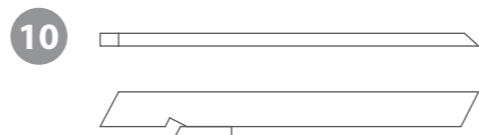
10 Right Roof Truss - 40x160x1308mm QTY 4 AI-12GAZHP0404RRT-V1
