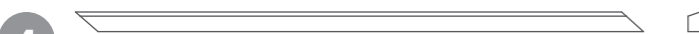
4 Top Truss Frame Right - 27x44x1612mm QTY 4 F2744-G-1612mm (1 x cut along profile, 2 x angled cuts right.)
