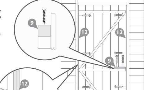
IMPORTANT: Pre-drill before fixing screws.
