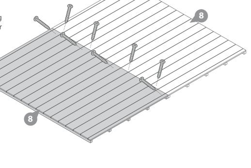
IMPORTANT: Pre-drill before fixing screws.
