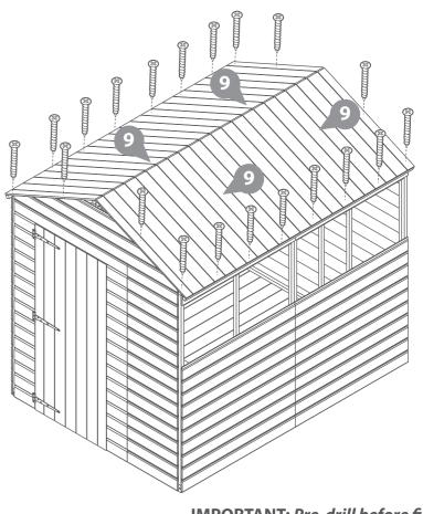
IMPORTANT: Pre-drill before fixing screws.
