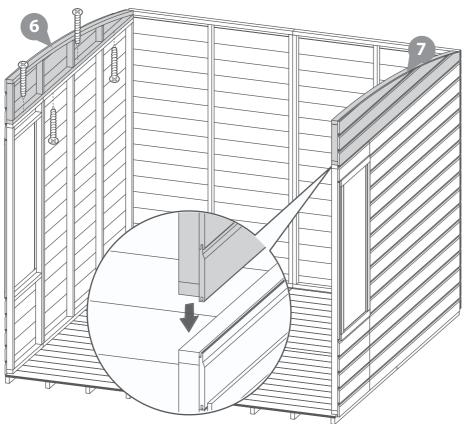
IMPORTANT: Pre-drill before fixing screws.
