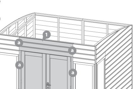
IMPORTANT: Pre-drill before fixing screws.
