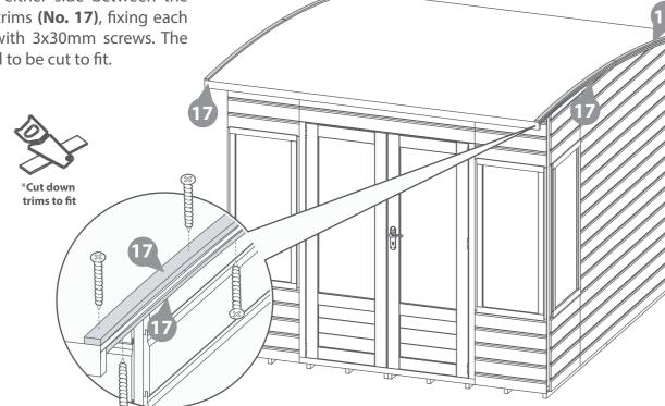
IMPORTANT: Pre-drill before fixing screws.
