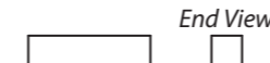
Truss Support Block - 44x44x176mm QTY 2 F4444-176mm *You may have more of this part than are required.
