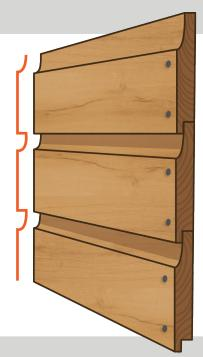
Shiplap cladding consists of multiple boards of timber which **creates a flush panel**. It also features a recess at the top of the individual boards which **helps water run-off**, offering protection against the elements. Not only is shiplap cladding **watertight**, but it also has the added benefit of being **airtight**, meaning belongings are much less at the risk of draughts and dampness.
